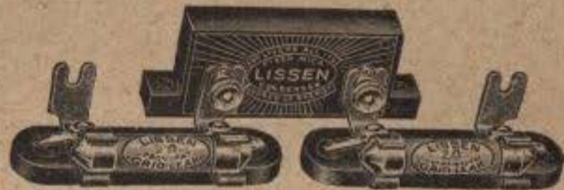
1. Shows the LISSEN COMBINATOR with LISSEN Fixed Condenser and LISSEN Fixed Resistances linked up to form a complete r.c. coupling unit for H.F. or L.F. amplification. The condenser is a .002, the resistance on the right can be a grid leak resistance of 2 megohms, and the LISSEN Resistance on the left is the anode resistance, which can be 1 megohm.
